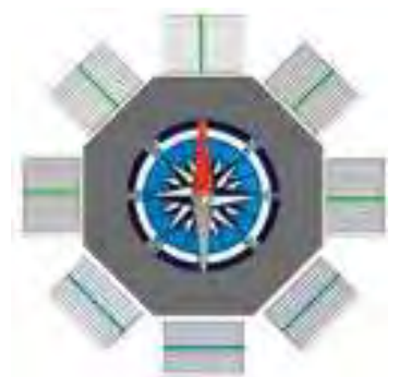
E-NE-N-NW-W: blades perpendicular to the wall. SW-S-SE: blades parallel to the wall.
